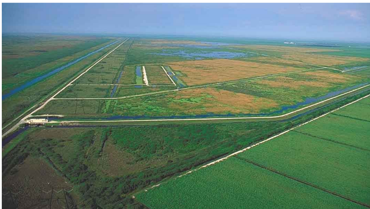
Figure 10: Aerial view of storm water treatment areas (STAs) and pumping stations next to agricultural sugarcane fields. The remaining natural Everglades are located to the left of the diked road and power lines. The STAs are used to reduce nutrient loadings and organic floc into the Glades (photo courtesy of the SFWMD).
