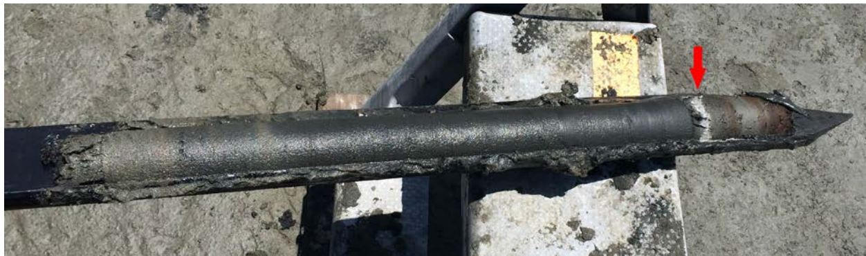
Figure 7: Core taken from feldspar plot using Russian corer. Arrow marks the location of the feldspar marker horizon, used to indicate the pre-augmentation marsh surface. Sediment above the marker horizon (to the left in the image) represents added sediment. Photo: A. Wagner, UCLA.
